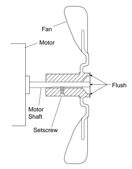
Figure 4 - Fan Cross Section
